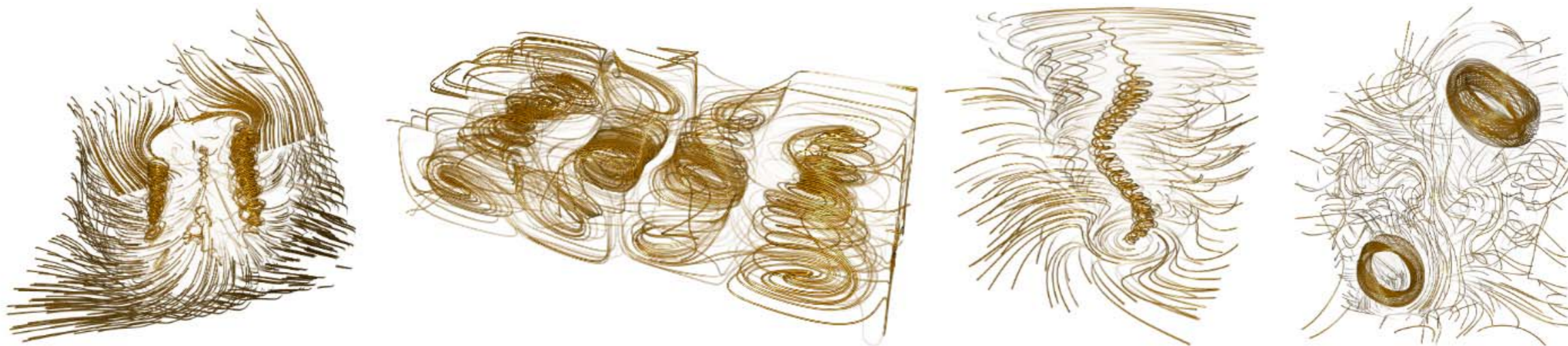
Figure 1: Applications of our interactive, global line selection algorithm. Our bounded linear optimization for the opacities reveals user-defined important features, e.g., vortices in rotorcraft flow data, convection cells in heating processes (Rayleigh-Bénard cells), the vortex core of a tornado and field lines of decaying magnetic knots (from left to right).
