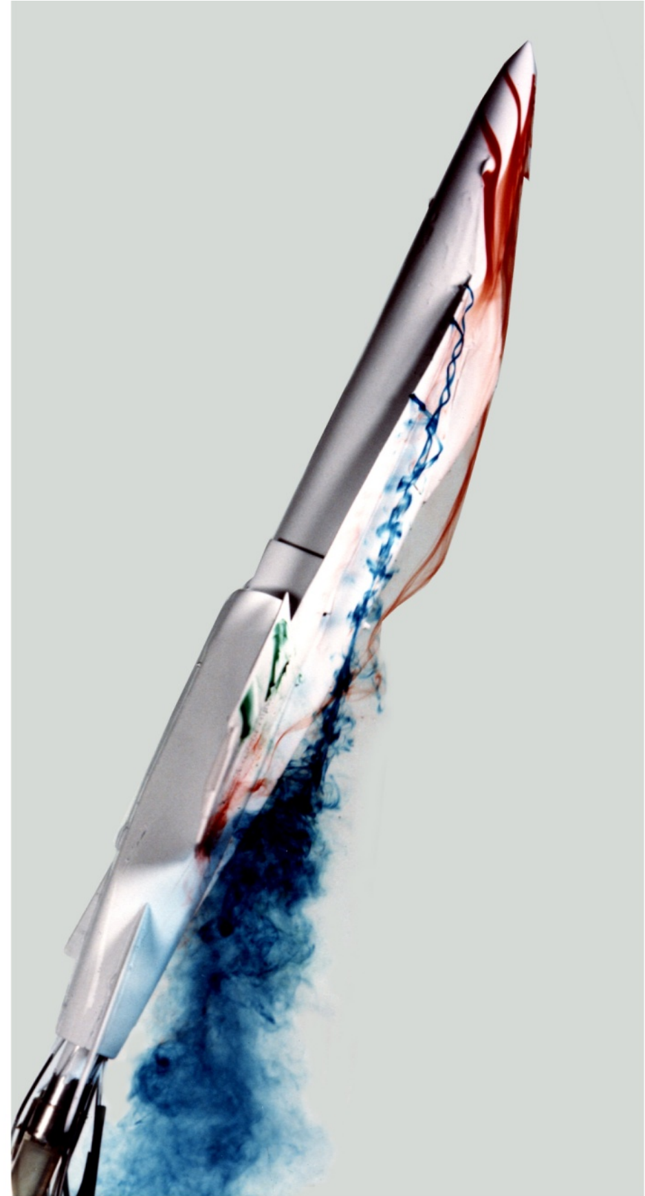
Dryden Flight Research Center ECN 33298-47 Photographed 1985 F-18 water tunnel test in Flow Visualization Facility NASA/Dryden
