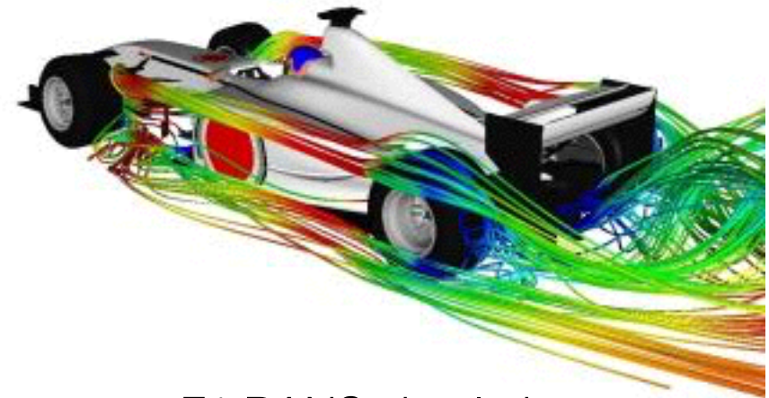
F1 RANS simulation http://www.symscape.com/blog/car-design-cfd
